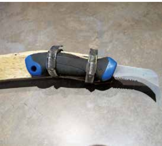
Fig. 10. A linoleum knife tied to a staff was used to cut the tarp in half to facilitate its removal during planting. Photo by Susan Lightburn.
